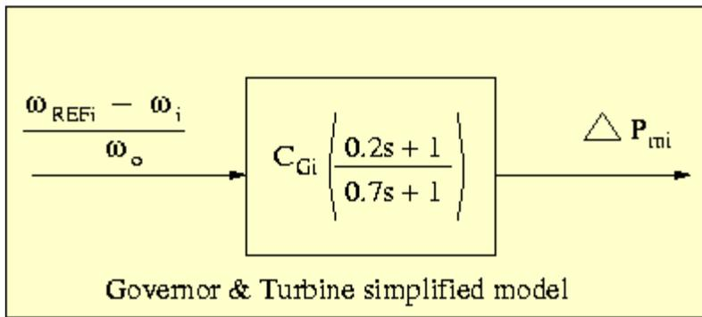
Assume that for both generators,  $P_{m0i} = 0.5$  and  $C_{Gi} = 20$ ;  $\omega_{REFi} = \omega_o = 2 * \pi * 50$
